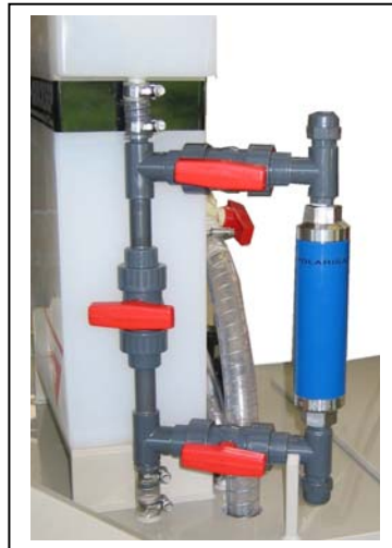
FM-Polarizer on coolant cleaner MINI-Quicksep
