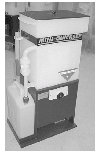
MINI-QUICKSEP 120 with 10 l oil tank.
